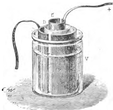
Fig. 4.—A Daniell's Cell. E = 1.07 volts.
