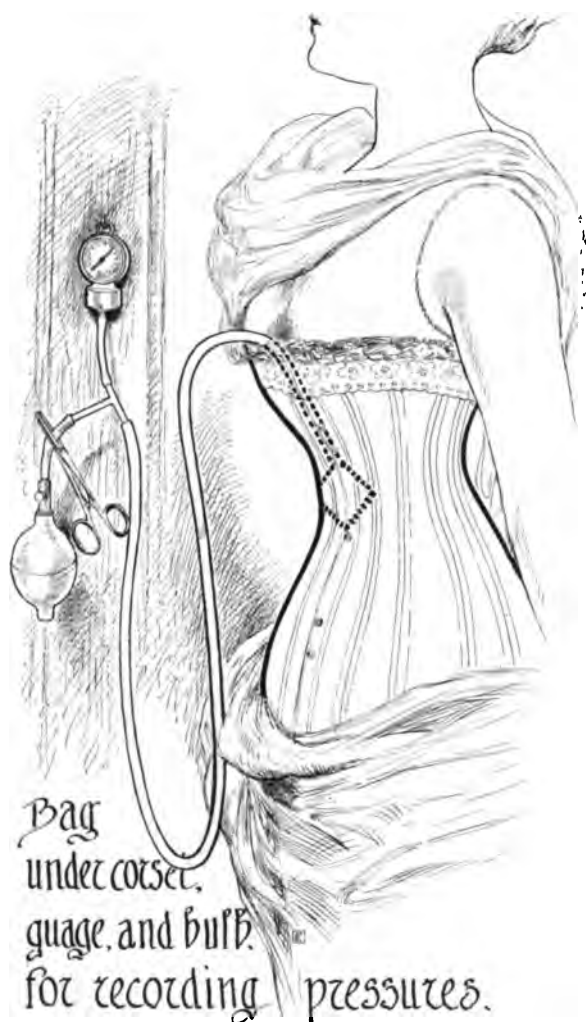
FIG. 31.—Pressure measurements. An aneroid (sphygmomanometer) hanging on the wall, is connected by tubing with a bag that is slipped under the corset.
