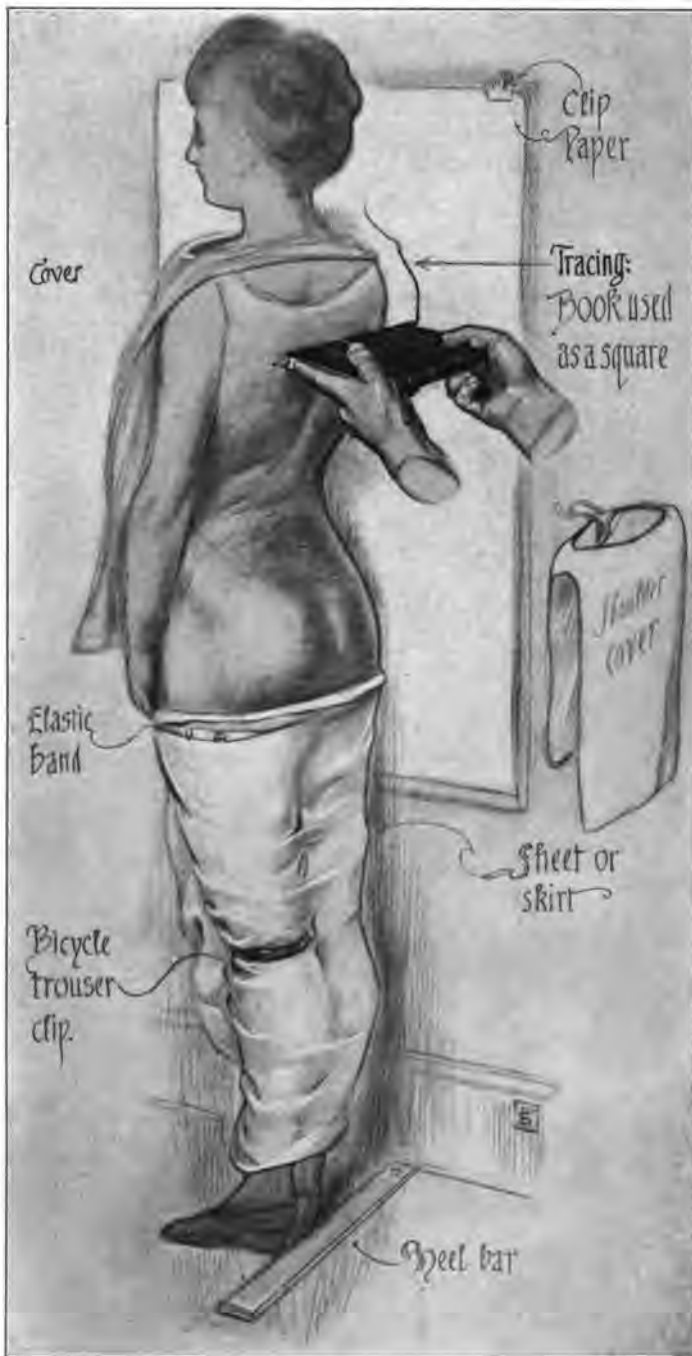
FIG. 35.—Simple method of recording outlines. Against a heel bar the subject stands. The paper is clipped to wall or drawing board. A pencil, held by elastics in the groove of a narrow book that acts as a square, follows the profile and makes a tracing. The knee action is shown by the snug sheet.
